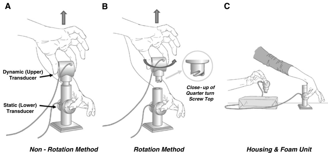
**Fig. 1** Schematics of the bimanual tasks examined in this study. **a** An example of the task performed with the Non-Rotation method; static and dynamic transducers are indicated. **b** An example of the task performed with the Rotation method. A quarter-turn rotation in the counter-clockwise direction was required when performing tasks
