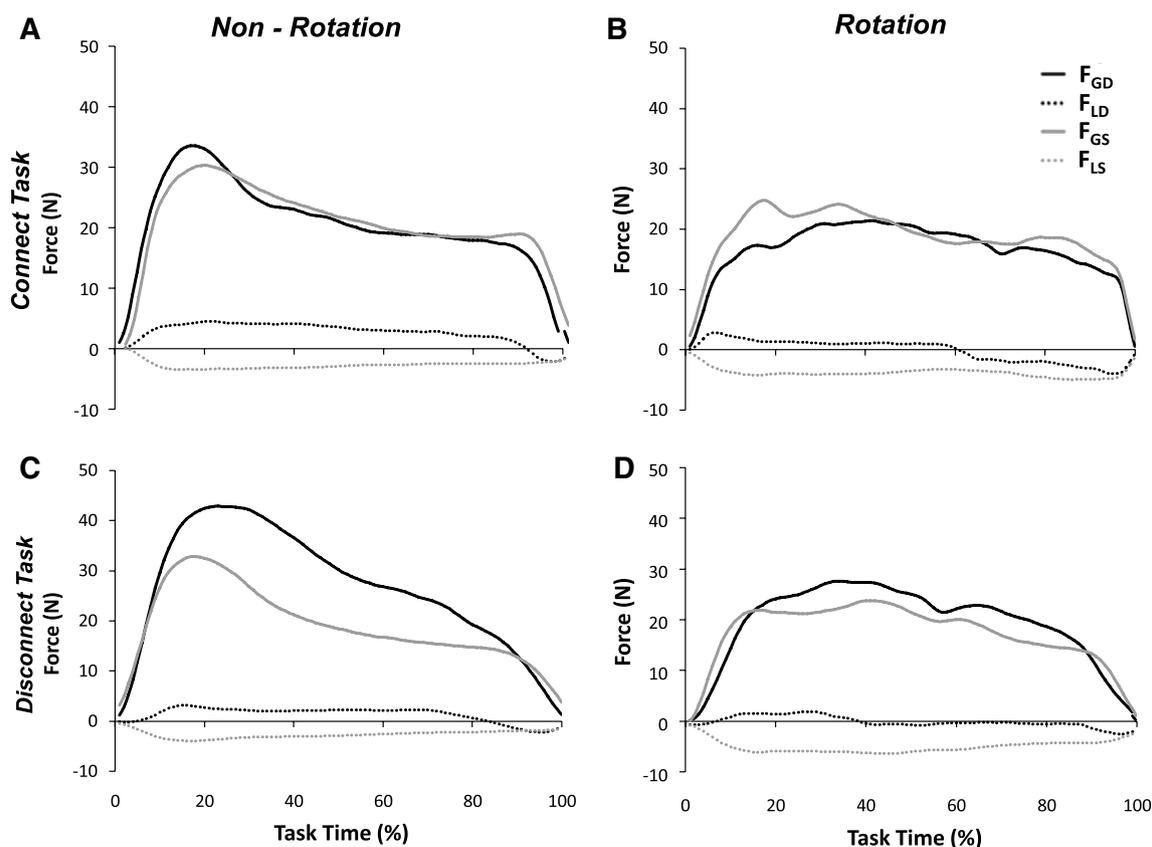
**Fig. 2** Average grip and load force profiles exerted of a typical subject in each of the four tasks examined with respect to movement time. Grip and load forces exerted on the dynamic (*upper*) transducer are denoted by  $F_{GD}$  and  $F_{LD}$ , respectively. Grip and load forces exerted on the static (*lower*) transducer are denoted by  $F_{GS}$  and  $F_{LS}$ , respectively. **a** Total grip and load forces exerted when the two trans-
