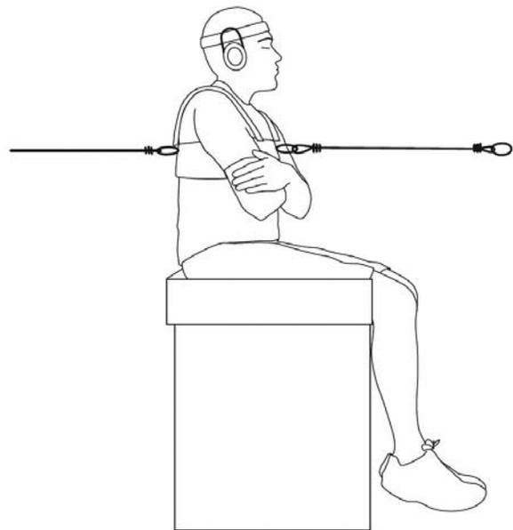
**Figure 1** — Illustration of subject sitting on experimental apparatus. Horizontal force perturbations were applied through one of eight cables attached to a harness worn about the chest.
